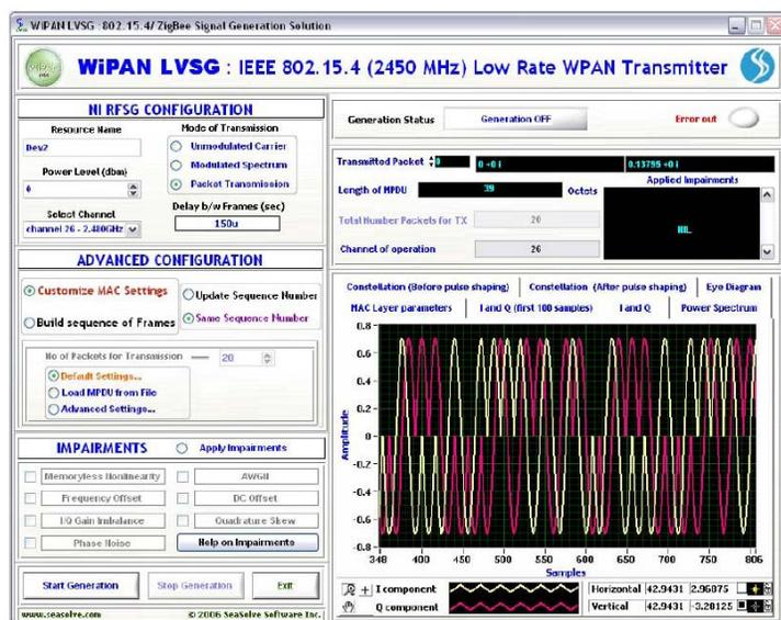
**Figure 3:** Main screen of the WiPAN LVSG solution, with a plot of transmitted IQ data
