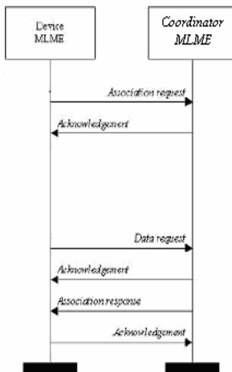
**Figure 5:** The diagram on the right shows a sample exchange of MAC messages defined in the 802.15.4 standard; WiPAN LVSG, as seen on the left, can emulate either a PAN device or coordinator in order to test the DUT's response to standard MAC commands
