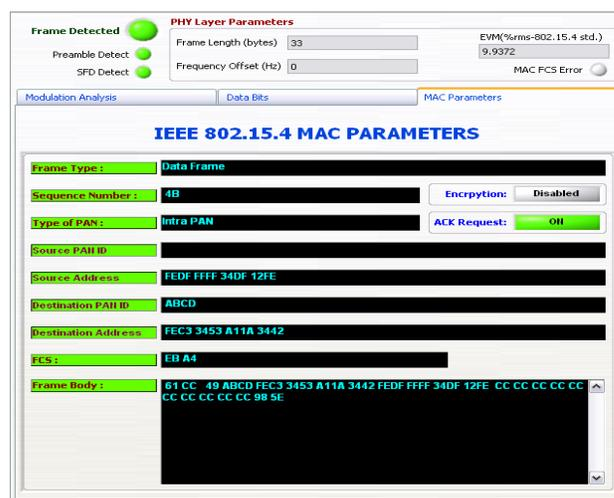
**Figure 9:** MAC demodulation of incoming data frames; notice the indicator LEDs above the plot area
