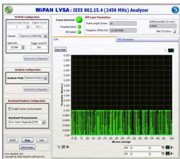
Figure 1: Checking transmitter EVM
