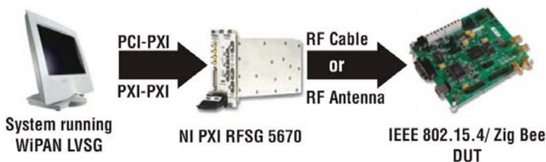
**Figure 4:** Setup to generate and transmit 802.15.4 signals to a WPAN DUT
