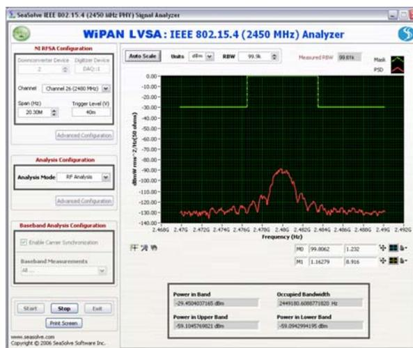
Figure 6: RF analysis of an 802.15.4 signal
